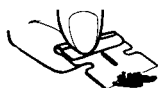
Do use a razor blade to remove excess burn-ons. Hold blade so entire edge is on cooktop at a 30° angle.
